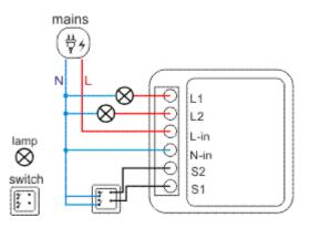
Note: The ZigBee Switch must be powered up by N and L wires
